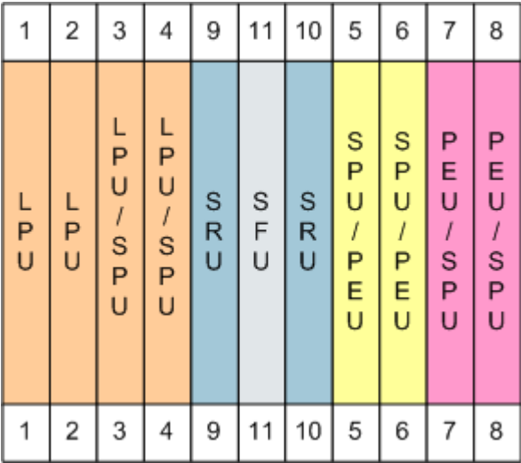
Figure 3-9 Layout of boards in the PGP-X8 subrack
